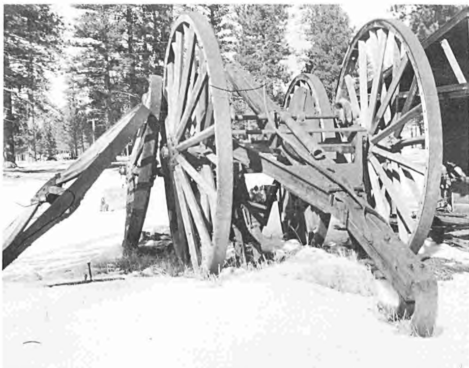
Equipment used in the early 1900's by Long-Bell. Slip tongue wheels. Wheels 12' in diameter.
