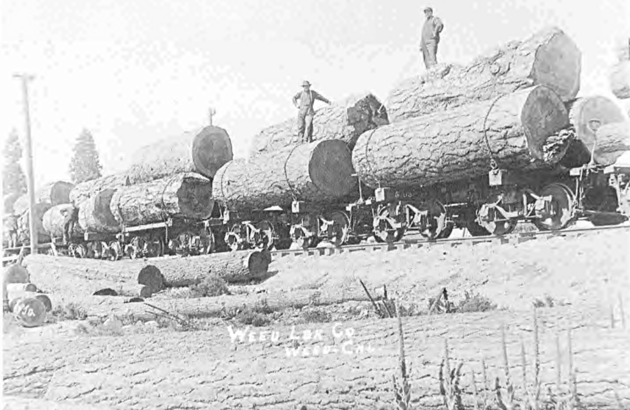
Loads of logs to be unloaded into mill pond. Russell logging cars in use before air brakes.
