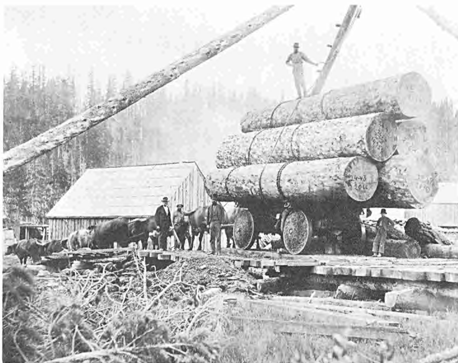
1896-1900 at Mr. Weed's logging operations near Black Butte. Oxen and wooden wheeled logging wagons were used. Loaded by a steam donkey engine.
